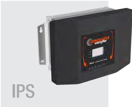
The **IPS** (Inductive Power Supply), converts the 50 or 60 Hz mains frequency into a high frequency allowing highly efficient power transfer. Charging requirements and other information coming from the Battery management system onboard the vehicle is taken up by the IPS and transferred in corresponding action.
