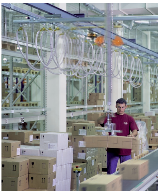
Easy packaging: C40 with Festoon System in a shipping warehouse
