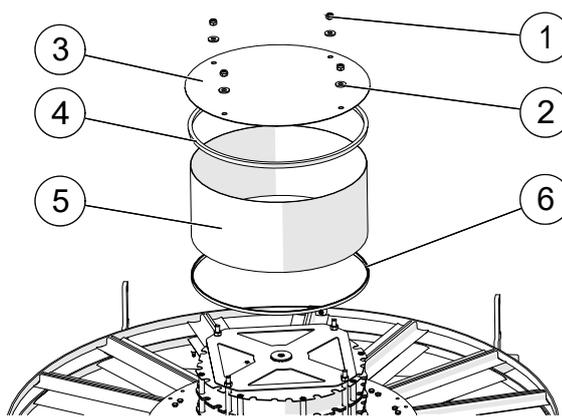
Fig. 2: Dismantle the Spring Housing
