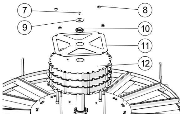
Fig. 3: Remove the Spring Cassette
