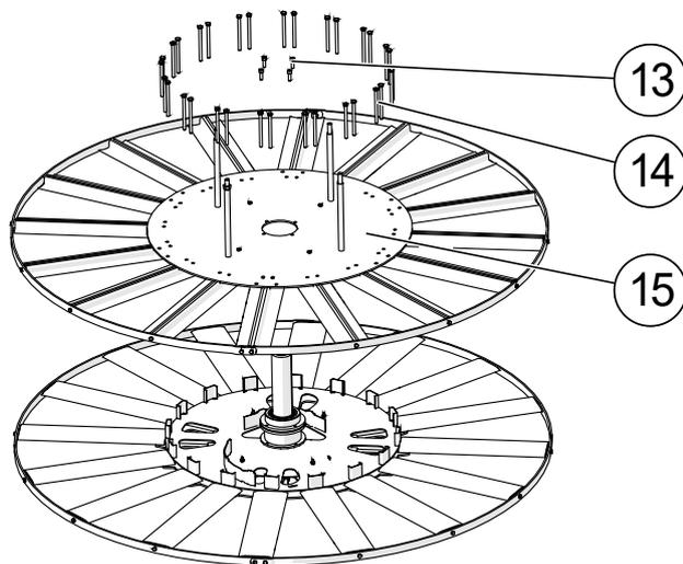
Fig. 4: Disassembly of the Spoke Wheel
