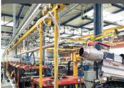
Jib boom, Equipment carrier, Balancers + Retractors
