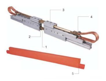
The expansion section consists of a sliding section inserted in a 6 meters long rail. A series of strips (1) maintains the contact surface and ensures electrical continuity.
