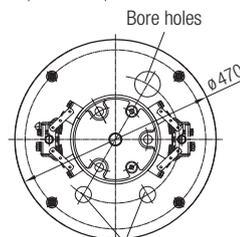
Bore holes in the floor panel intended for the following screw connections:
