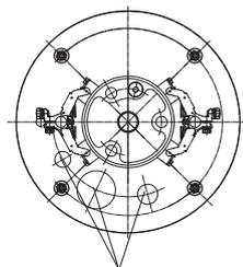
Bore holes in the floor panel intended for the following screw connections:
