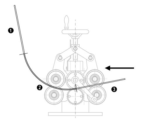
4. **Loosen** the spindle, pull the rail out.
