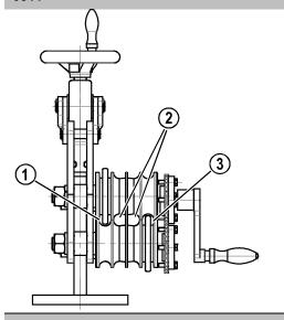
Bending groove for vertical curves with the engagement slot inside.
