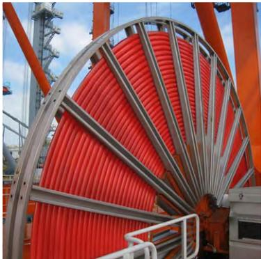
The **Monospiral Spool** wraps the cable in the same plane and prevents the cable from twisting. It is your guarantee of a longer cable life.
