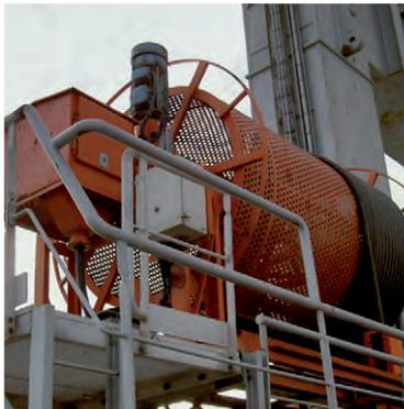
**Level Wind Spools** are designed to accommodate cables that are 1,000 meters or longer.
