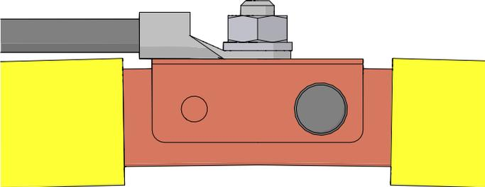
8. After the cable was connected, put the feed cap over the feeding point and consider the direction for the cable.
