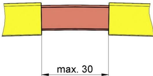
3. Put the U-plate on the right position and drill a hole with  $\varnothing = 3.1$  mm (one hole on each side with a staggered arrangement).
