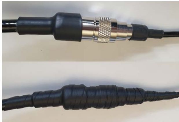
Fig. 93: Connection point sealing
