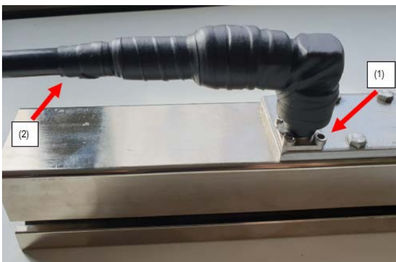
Fig. 24: Wrap socket and cable with adhesive tape
