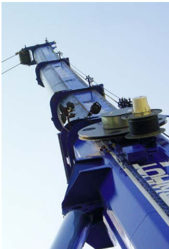
Slip ring assembly in construction machine
