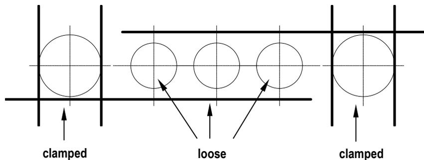
Fig. 30: Schematic diagram of preparation for installation of round cable clamps
