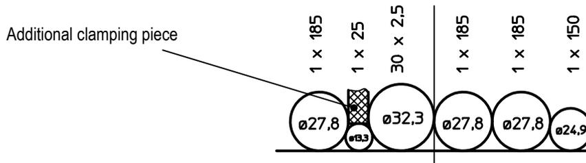
Fig. 26: Using clamping pieces
