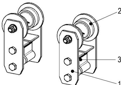
Fig. 14: Running gear
