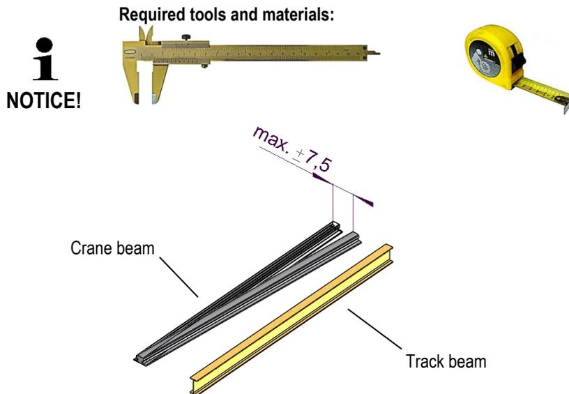
Fig. 7: Poor horizontal alignment between the crane beam and the track beam
