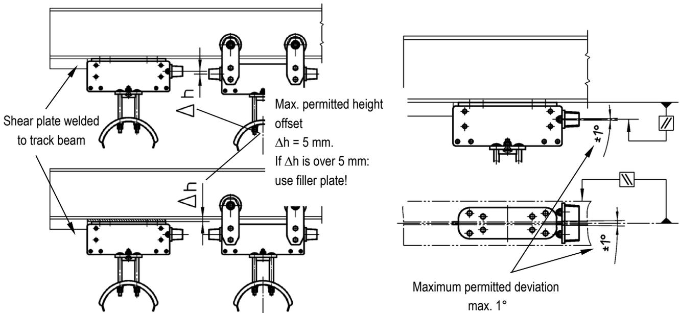
Fig. 24: Mounting the end clamp
