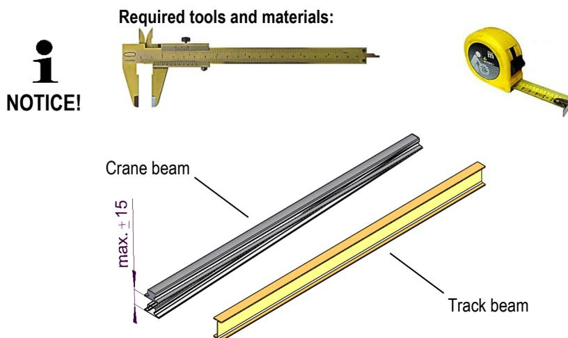
Fig. 8: Poor vertical alignment between the crane beam and track beam
