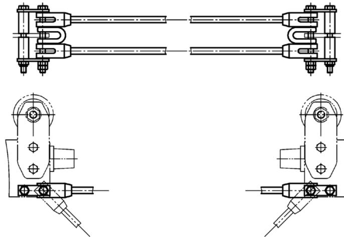
Fig. 34: Damping device with 2 shock cords
