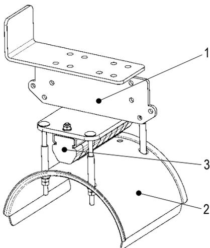
Fig. 13: Towing clamp
