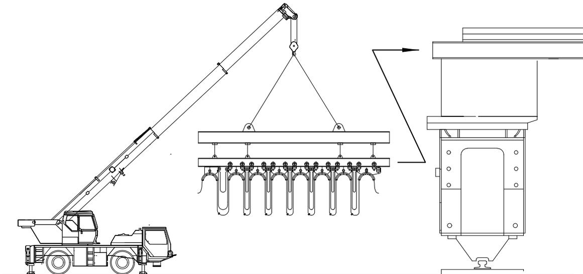
Fig. 21: Mounting a pre-assembled festoon system
