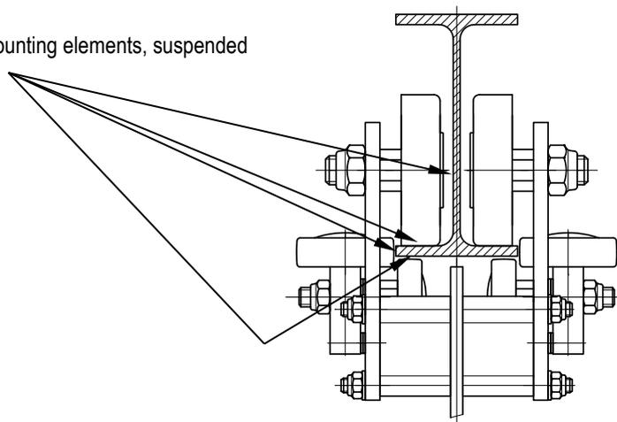
Fig. 2: Use of even welded track beams
