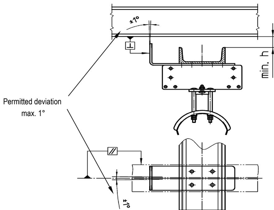
Fig. 22: Mounting a towing clamp
