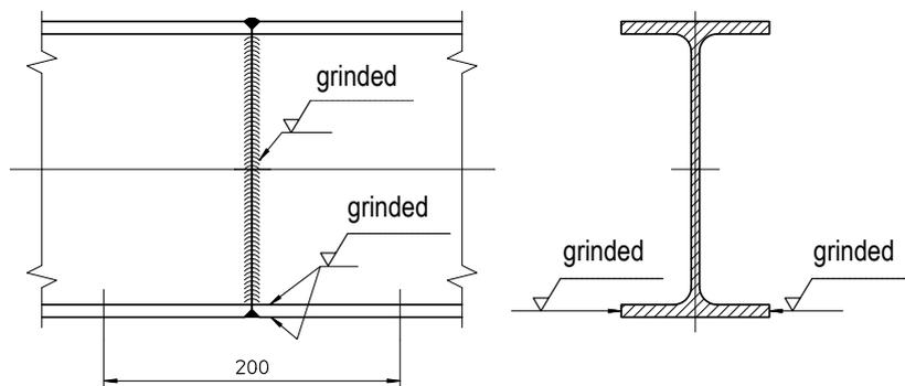
Fig. 1: Smoothing of welded track beams
