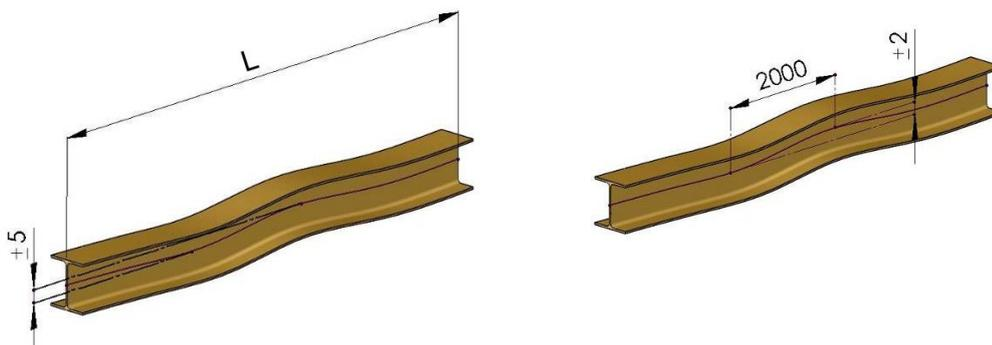
Fig. 6: Vertical deviation of track beams
