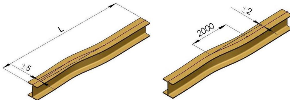
Fig. 5: Horizontal deviation of track beams, L = total length
