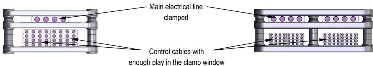
Fig. 32: Installing flat cable clamps
