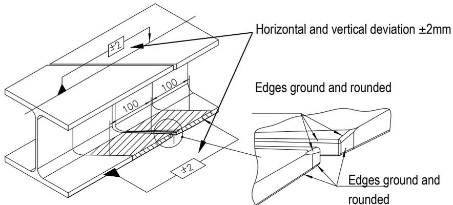
Fig. 4: Girder joint for non-welded track beams
