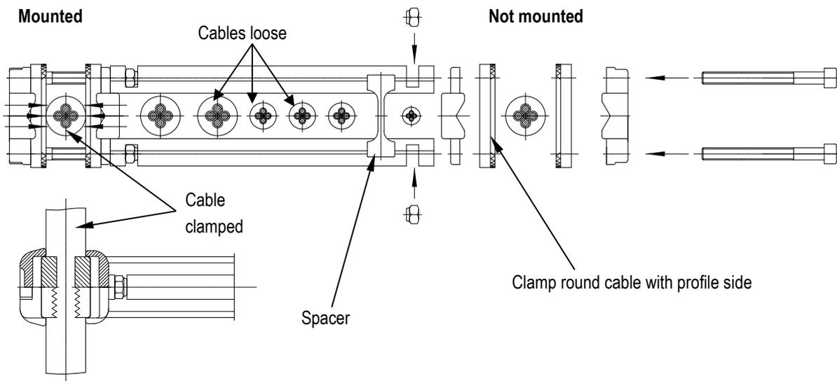
Fig. 29: Mounting round cable clamps
