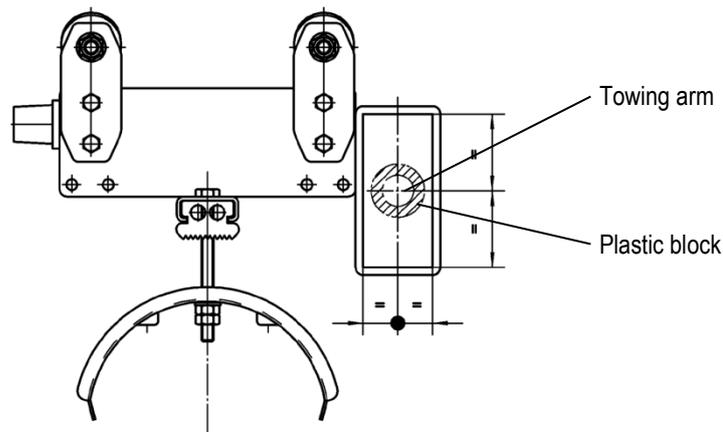
Fig. 23: Orientation of the towing arm
