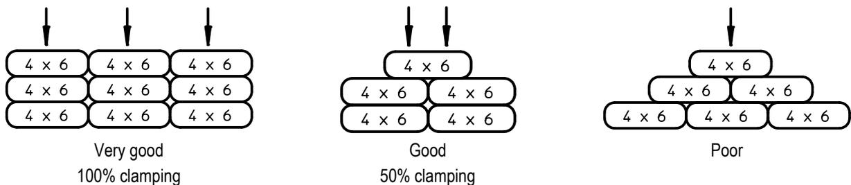
Fig. 28: Arrangement of flat cables
