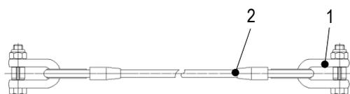
Fig. 16: Towing rope
