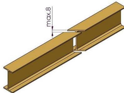
Fig. 3: Girder joint for non-welded track beams
