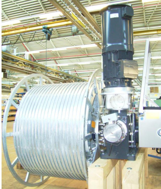
EB reel body for defined cable winding
