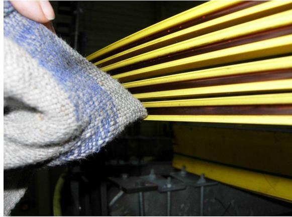
Figure 11: Angle for cleaning the lower area
