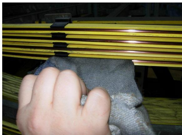
Figure 9: Also remove dirt from the hanger clamps
