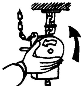
To increase the tensile force, the spring housing is rotated in the direction of the cable pull.
