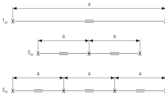
$a$  = distance between anchor points  $\rightarrow$  arranged symmetrically as much as possible
