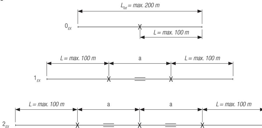
$a$  = distance between anchor points  $\rightarrow$  arranged symmetrically as much as possible
