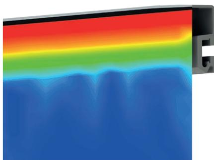
Electromagnetic emissions in the slotted waveguide
