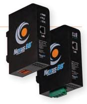
**Nexus BB** is a powerline communication system for Ethernet with a data rate of up to 100 Mbit/s, using the phase lines of the AC or DC power transfer on the conductor rails supplying the shuttle, to ensure communication between higher-level control and the vehicle. **Nexus BB** acts as a virtual Ethernet cable and can connect several shuttle levels to one stationary transceiver, provided these are connected to the same power supply.
