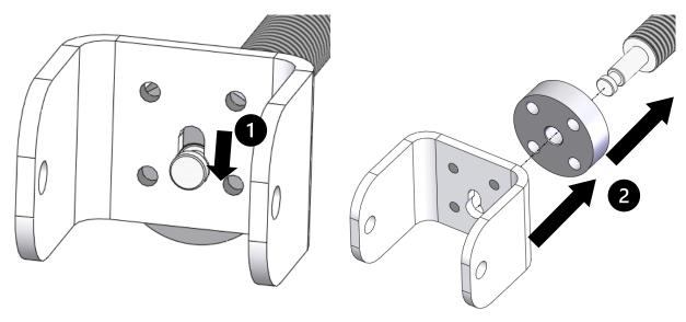
The roller itself has been hidden in the picture for better visibility. It is not necessary to disassemble the roller.
